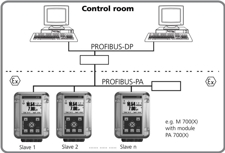
Electrical connection between module and PROFIBUS PA is in accordance with the PROFIBUS Guideline, Order No. 2.092 ([www.profibus.com](http://www.profibus.com)).
